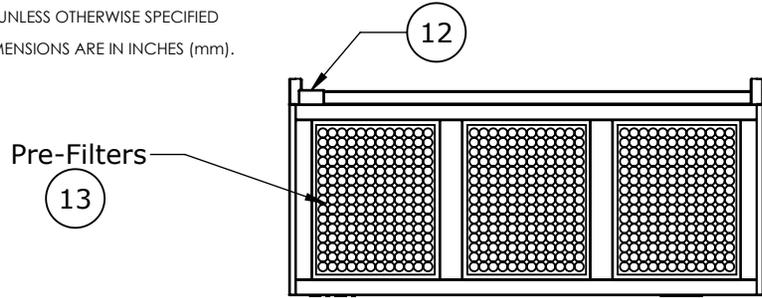
Prefilters can be relocated to the front or back of unit. Leave minimum of 4 inches of clearance from filter face
