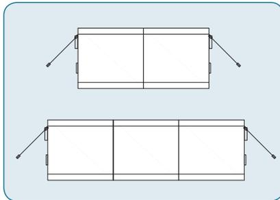
Tunnels are commonly used for “continuous flow” cleaning. Both 90-degree and straight-through air showers can be combined to form the tunnel configuration.
